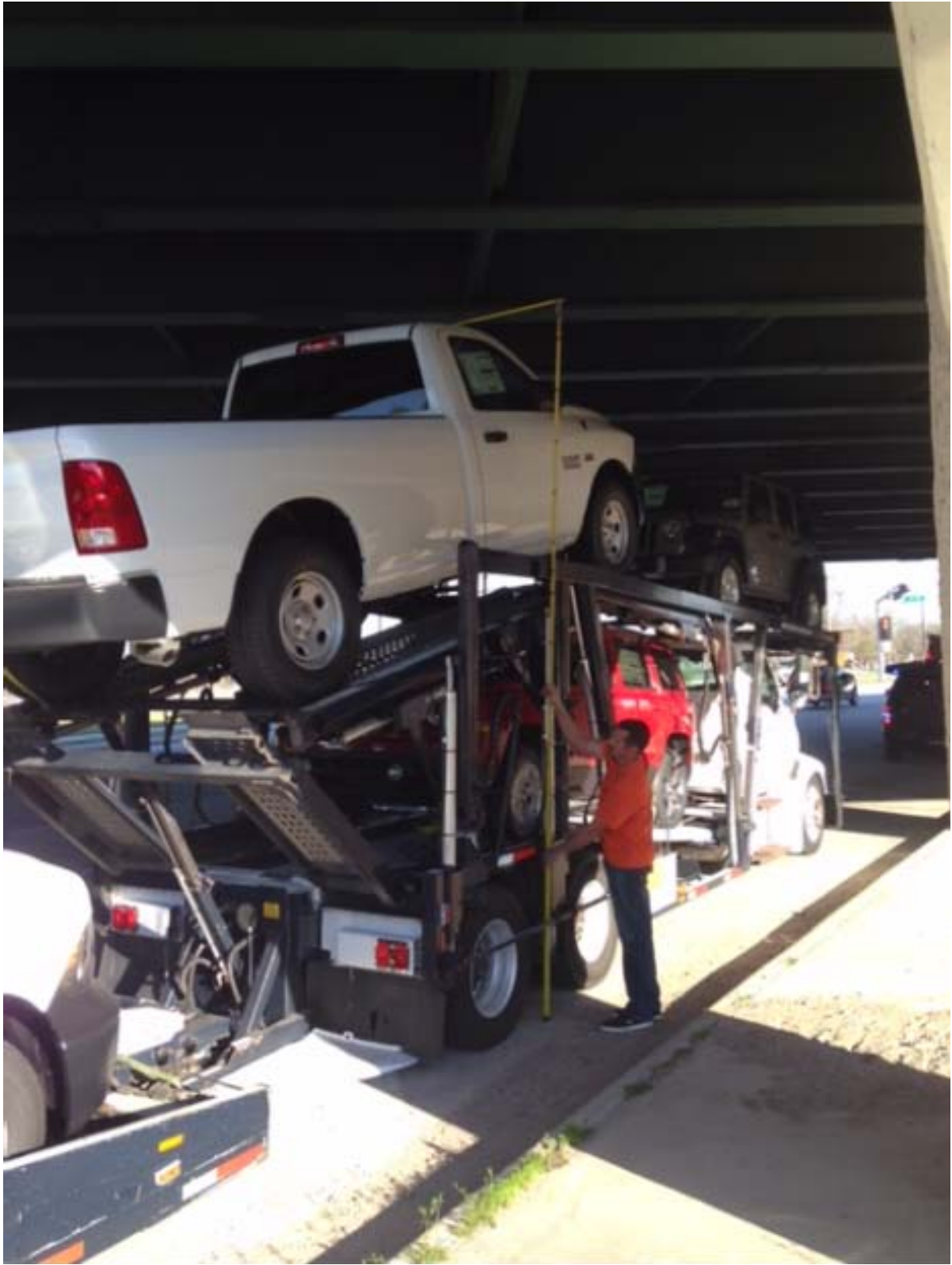
Figure 3. Vehicle 2 Measured for Overheight Status (Source: HPD TEU)
